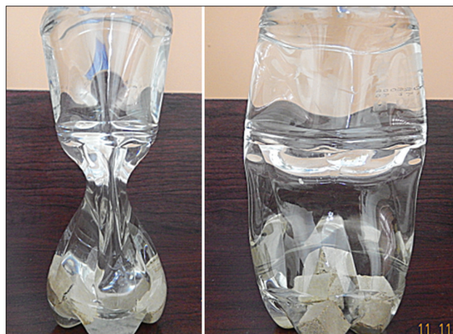
Figure 31: Polyethylene terephthalate (PET) bottle with drinking water and melanin impregnated in silicium (bottom). After few days, PET bottle deformation is evident
