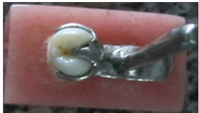
Figure 2: Cobalt–chromium Aker clasp and the framework with the testing model
